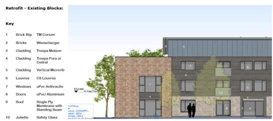
Figure 7 materials to Existing and New build blocks
